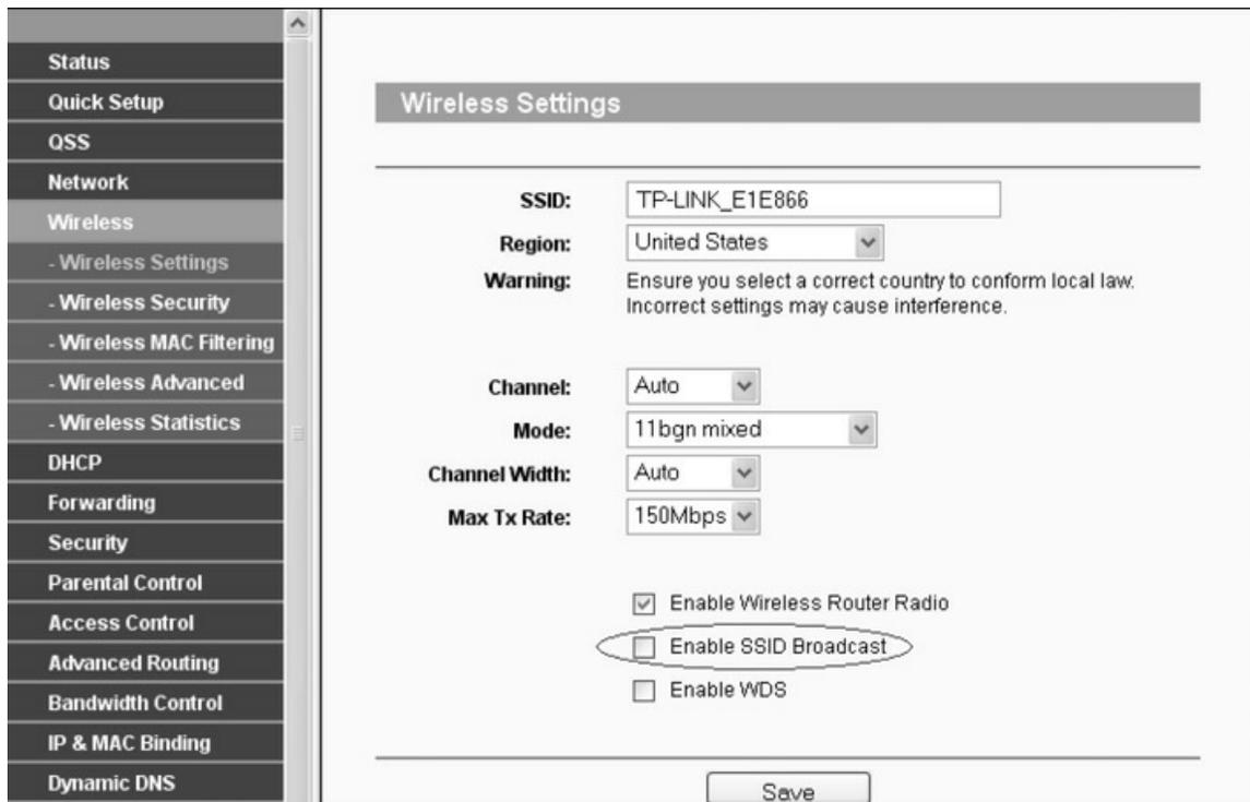
Figura 9.1 – Desabilitando o checkbox Enable SSID Broadcast.
